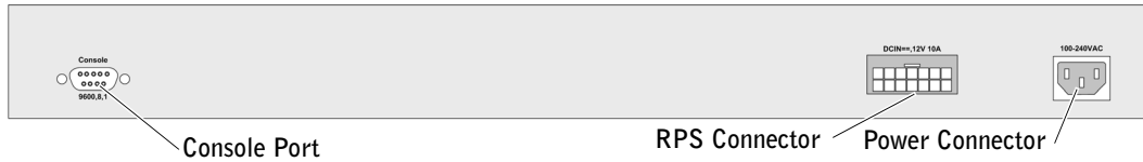
Figure 2-2. PowerConnect 3424 Back Panel
